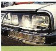
**Above:** The headlights of Citroen Maserati could turn along with the steering wheel. This smart detail design was a design feature of Citroen.
